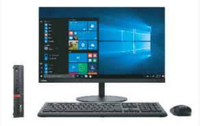
ThinkCentre M920 Tiny — Spacesaving form factor starting at 2.9 pounds that integrates quickly with the Lenovo ThinkCentre Tiny-in-One for completely modular, all-in-one computing. Configured with an 8th Generation Intel<sup>®</sup> Core<sup>™</sup> i7 processor and up to 32GB DDR4 memory.
